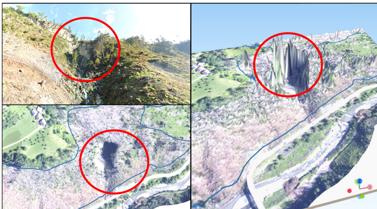
Figure 11: particular of an error in the restitution of the CHM due to a data acquisition problem that can occur along the escarpments
